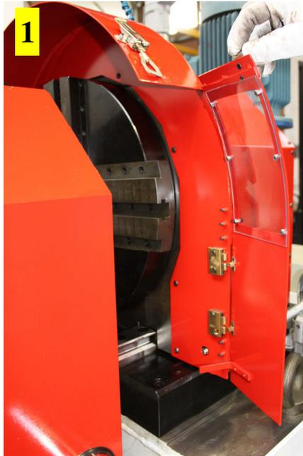
1) Open the lock and unhook the side door as shown in the above picture.
