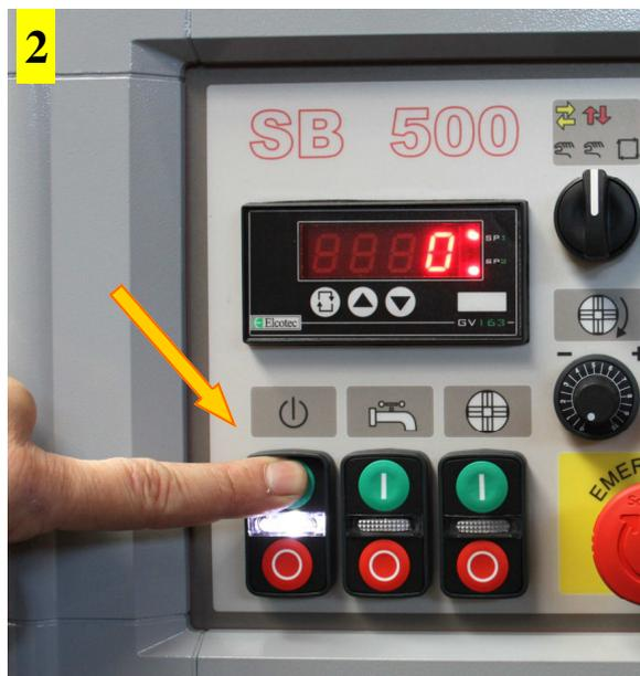
2) Press the green button on the control panel (reload button), the controls will be enabled.
