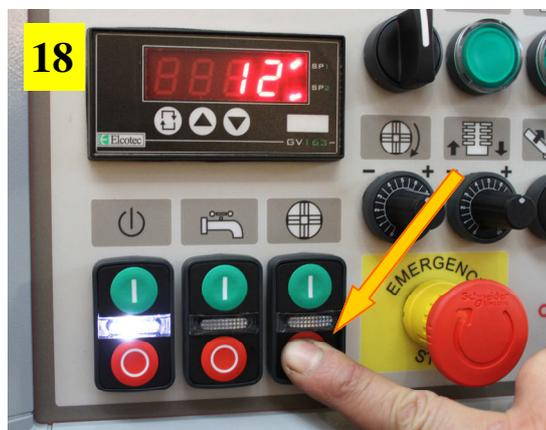
15) Press the green button shown in the picture (**MAIN START/STOP SWITCH**), per to enable the controls on the control panel.
