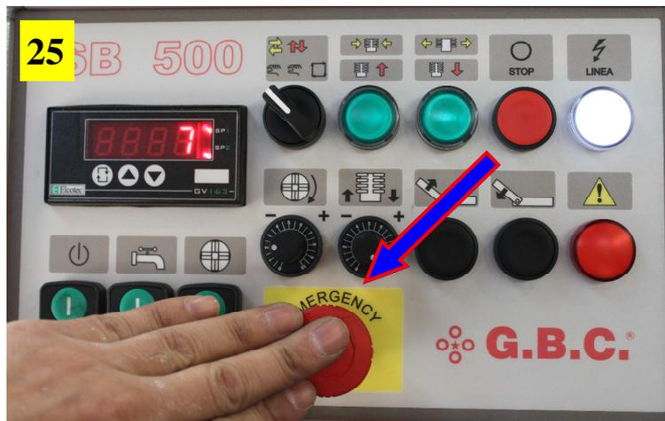
25) In case of an emergency press the red emergency button. The machine will cease any operation instantly.
