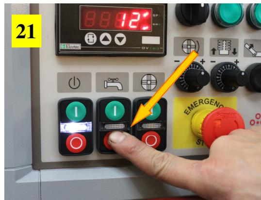
19) Press the green button as shown on the picture #19 (**COOLING PUMP START STOP**), to activate the pump.
