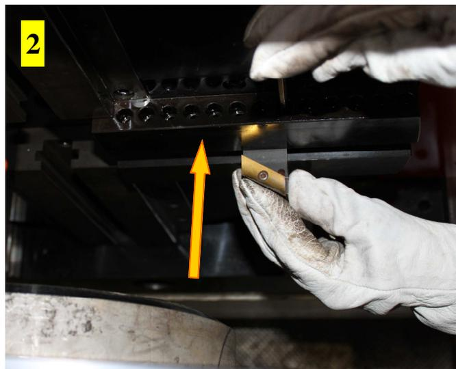
2) Get the selected tool and slide it in the mandrel slot making sure it is abutted to the back wall and move it in correspondence of the pipe wall as shown in the above picture, then fasten the grub screws to lock the tool in place.
