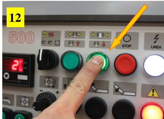
11) Ensure the switch (**Locking System/ Head Forward/ Automatic**) to be oriented on pipe locking function (**yellow arrows**) as shown in the picture.
