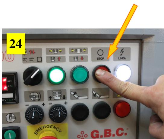
24) The AUTO cycle can be stopped at anytime by pressing the red button as shown in the above picture.
