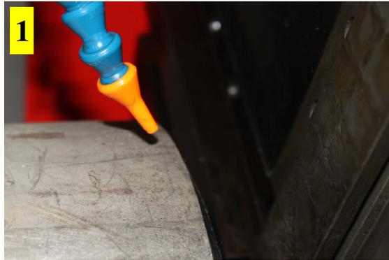
1) Position the nozzle of the cooling system right on the pipe edge as shown in the above picture.
