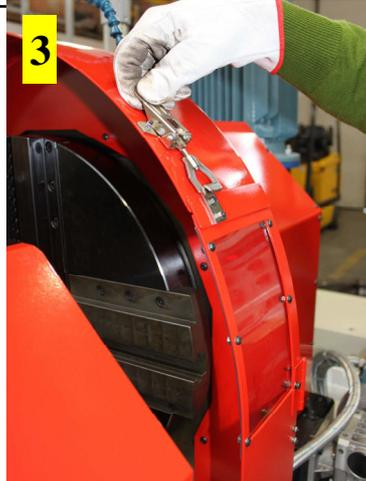
3) Once the tools are in position close the side door and hook the lock.
