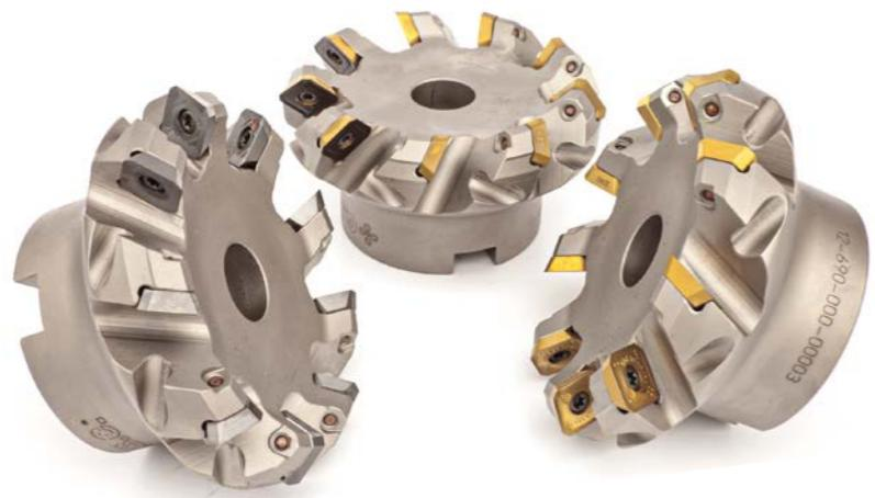
*The face mill equipped by every machines (with the exception of the Basic Edge 50), has 9 slots and can be fitted with different insert typology depending by the material you need to work (carbon steel, stainless steel, duplex, super duplex, inconel, aluminium, etc.). Every insert has 4 cutting edges therefore you will be able to use it for 4 complete working cycles.*
