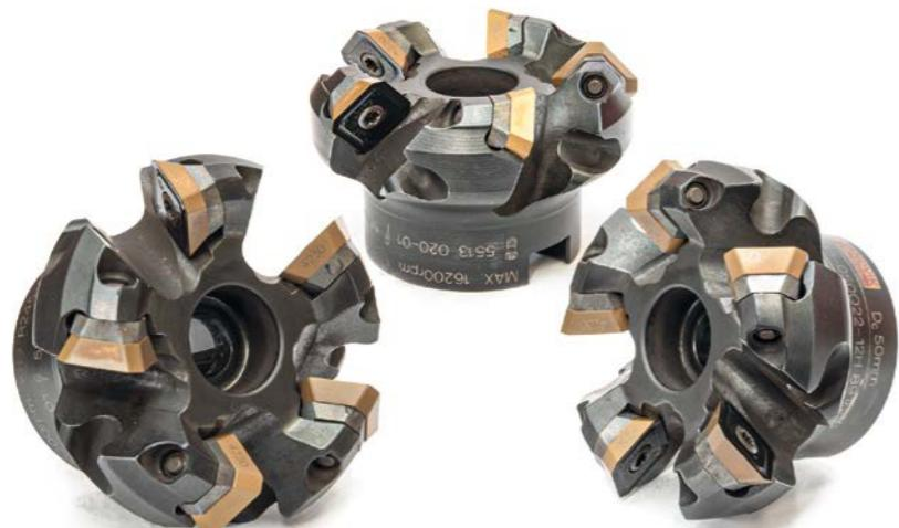
*The face mill equipped by Basic Edge 50 has 5 slots for inserts and, like the face mill for the other models, can be fitted with different insert typology depending by the material you need to work (carbon steel, stainless steel, duplex, super duplex, inconel, aluminium, etc.). Every insert has 4 cutting edges therefore you will be able to use it for 4 complete working cycles.*
